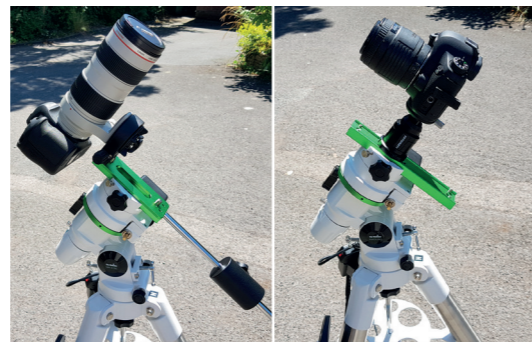
▲ Stripped-down versions of the mount, one with an L-bracket (left), the other with a ball head (right)
